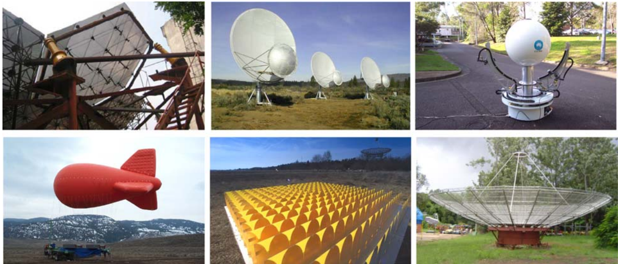
Figure 4. SKA technology prototypes. At left are components for large reflectors. The upper panel shows a prototype deformable surface for the FAST demonstrator while the lower panel illustrates a test aerostat for the suspended-feed LAR concept. The middle panel shows three 6 m dishes of the Allen Telescope Array (upper), together with a patch of an aperture array demonstrator based on Vivaldi-notch end-fire elements (lower). At upper right is a 0.9 m Luneburg Lens with a two-arm feed translator. The lower right panel shows a prototype 12 m dish constructed using a mesh surface and pre-loaded radial members.
