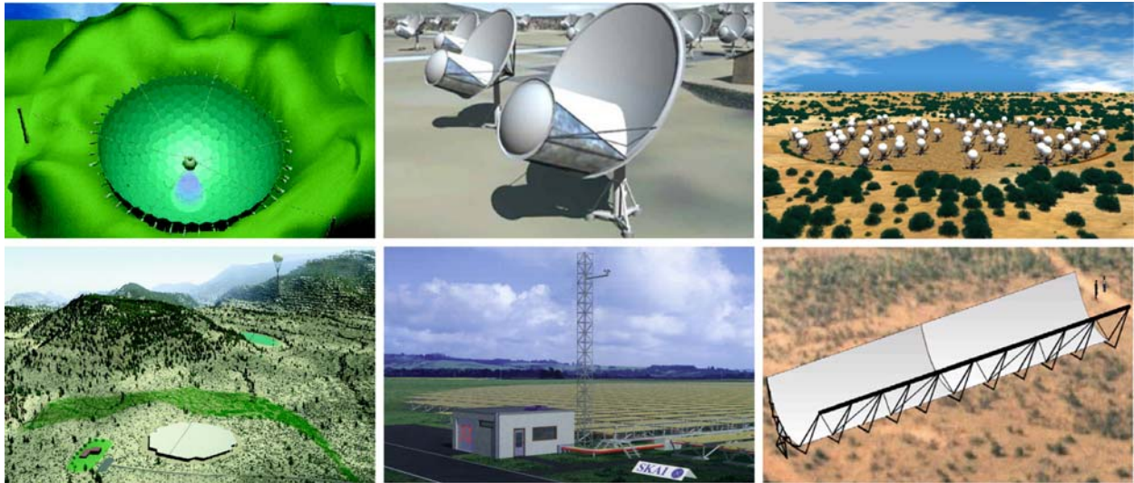
Figure 3. SKA concept visualizations. The left panel shows two large adaptive reflector ideas, one based on a 200 m diameter Arecibo-like spherical reflector (upper), the other using a much flatter reflector and an aerostat-mounted focus cabin. The middle panel (upper) shows offset paraboloids, the proposed 12 m versions being similar to the 6 m Allen Telescope Array antennas shown; the lower illustration shows an SKA station using aperture arrays. The right panel (upper) shows a station based on 64 x 7 m diameter Luneburg Lenses; the lower visualization is of a station employing a single 110 m x 15 m cylindrical reflector. The concepts originate in China, Canada, the USA, Europe and Australia (both right hand panels). Not shown is a 12 m symmetrical paraboloid concept proposed by the Indian SKA group.
