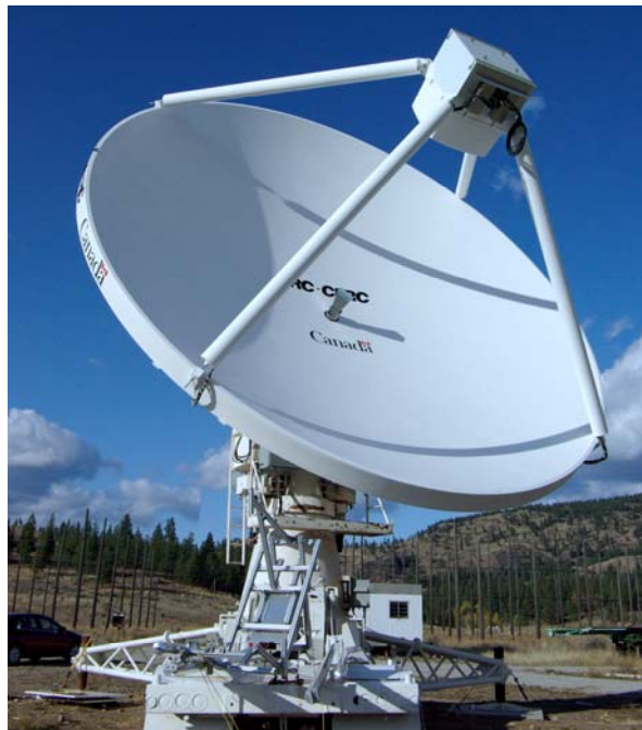
Figure 4 Mk2 Reflector on Positioner with PHAD in place.
