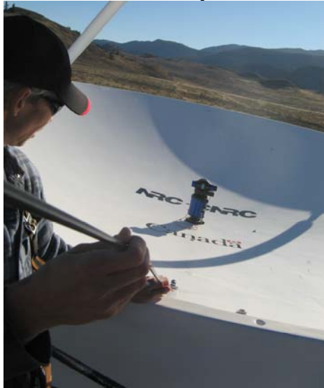
Figure 2 Measuring reflector surface with laser tracker.
