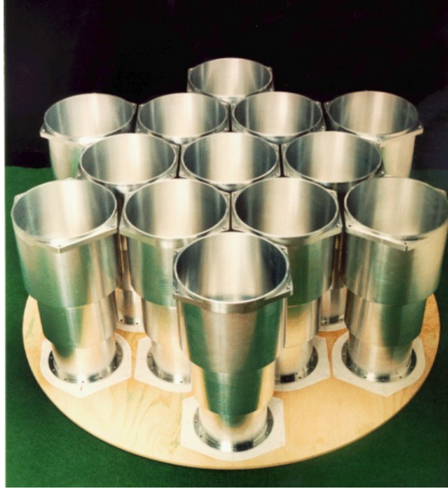
Figure 1: The horn array of the Parkes Multibeam Receiver.
