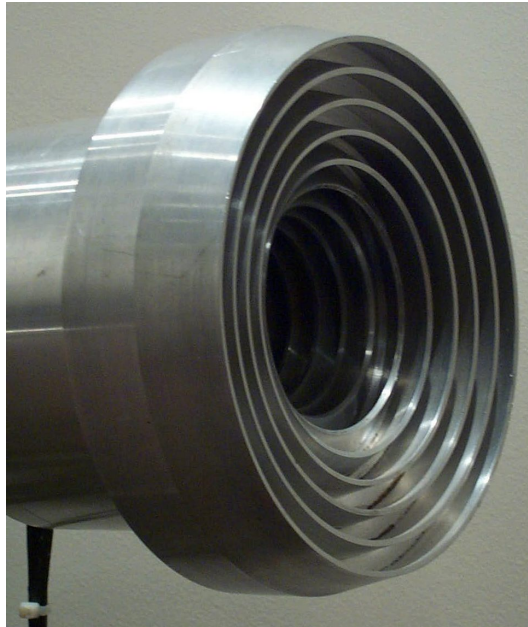
Figure 2: A wide-band corrugated feed similar to that described by Thomas et al. [9]. Notice that the horn flare is curved rather than linear as is the usual case with corrugated horns.
