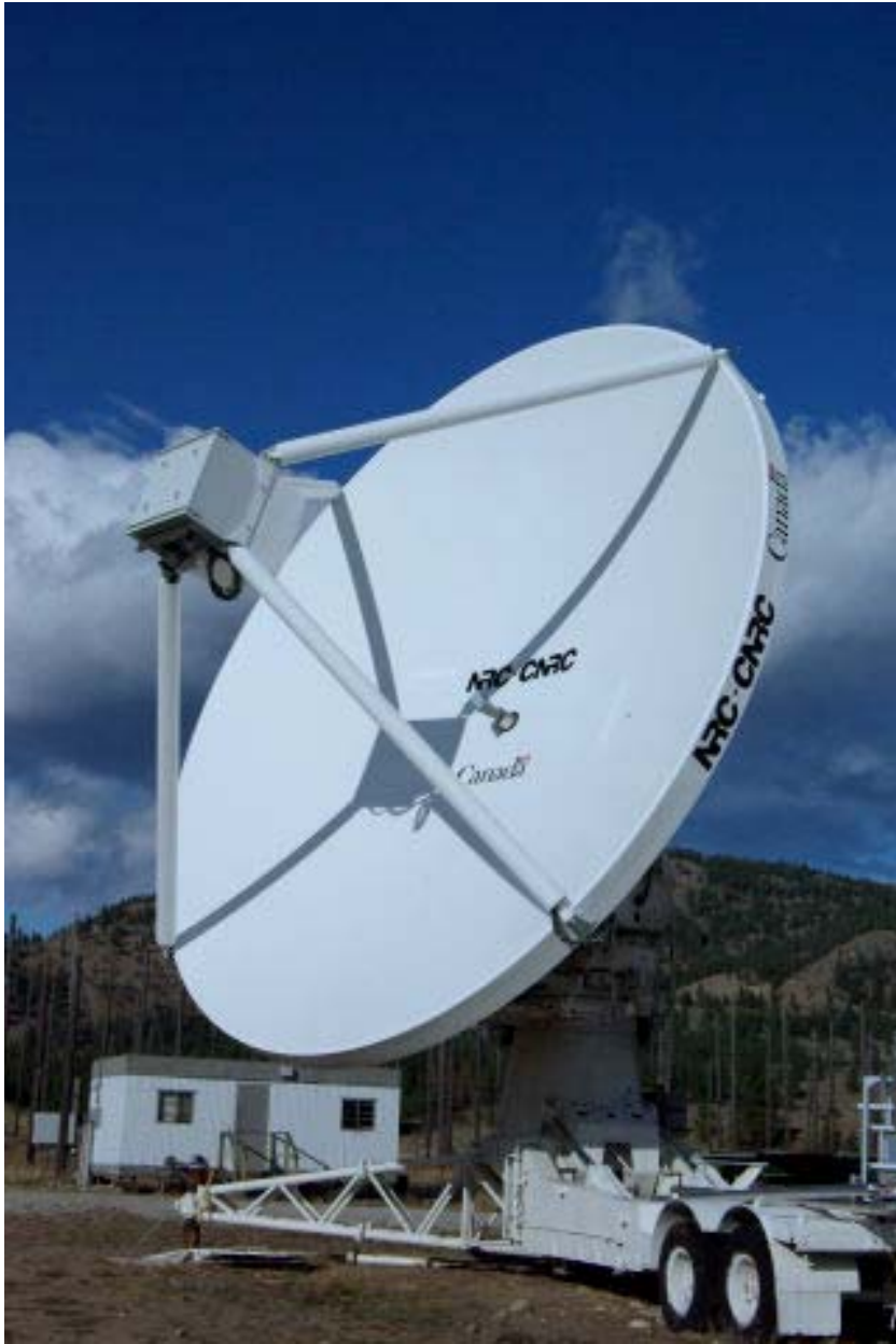
Figure 3. The Mk2 antenna complete with the 196-element PHAD array, mounted on September 26, 2008. PHAD is now undergoing on-the-sky testing.
