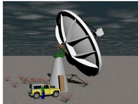
*Figure 4. Rendering of a 12-m CART antenna currently under development at HIA DRAO.*
