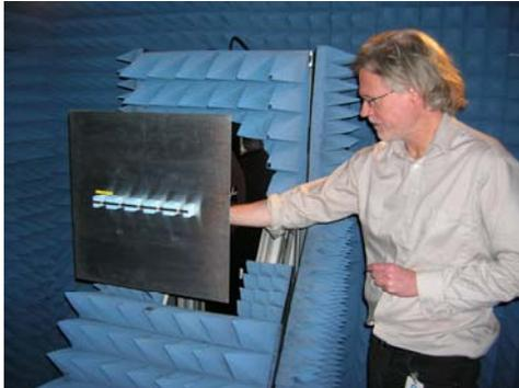
Figure 3: Stuart Hay testing the 5x1 prototype linear connected array.
