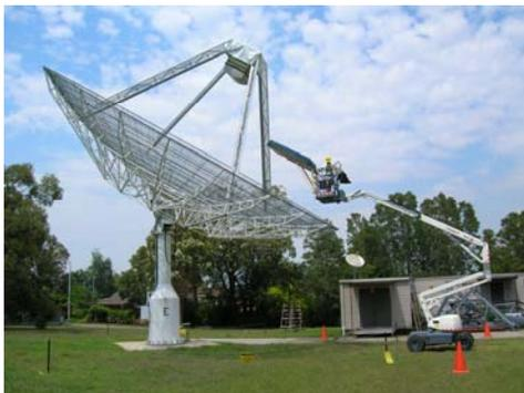
Figure 1: Noise measurement of the ATNF-Marsfield dish with the ASTRON THEA tile used as a phased array feed.
