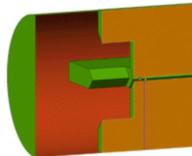
**Figure 32.** A cut through the back section of the OMT. The ridges are excited by passing a coaxial cable through the ridge and connecting the centre conductor to the opposite ridge. This high-precision pin was made by Thys Willemsse, a watchmaker from On Time Watch Services in Cape Town.
