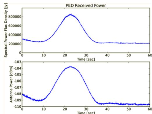
**Figure 35.** Calibrated drift scan results through the sun.
