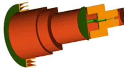
**Figure 31.** Cross-section of the full assembly, showing the horn, radome and quad-ridged OMT. While the model looks simple, it is electromagnetically complex. It required numerous runs of our in-house CEM software package, FEKO, on a SGI Altix 450 to develop the required insight into the physics of the structure.
