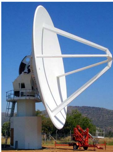
**Figure 30.** The MeerKAT prototype on site with all major mechanical components installed. The prototype is at the Hartebeesthoek Radio Astronomy Observatory in South Africa.
