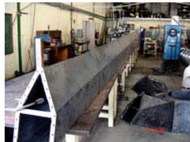
**Figure 23.** Manufacturing of the feed support legs
