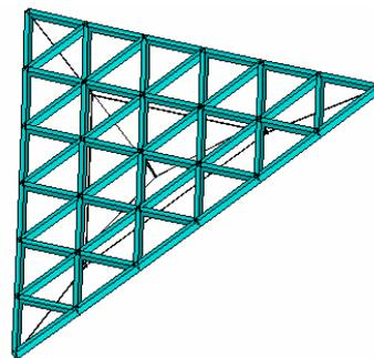
**Figure 10.** Reflector panel layout in a beam string structure
