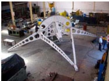
**Figure 21.** Assembly of the backing structure
