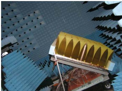
**Figure 18.** The EMBRACE prototype tile under test in the ASTRON anechoic chamber.
