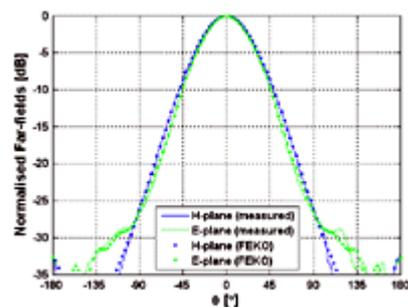
**Figure 34.** The measured far field pattern (shown here at 1 542 MHz) agrees very well with the values predicted using FEKO. These patterns will result in about a -13 dB edge taper on the 15 m prototype meerKAT dish.
