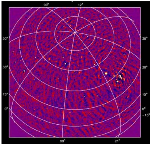
**Figure 19.** First deep, wide-field image made with the first LOFAR stations at a frequency of about 50 MHz. The angular resolution of the image is about 0.5 degrees. The image is centred on CasA, the brightest radio source in the sky, which was removed from the image. The image was obtained by Ger de Bruyn (ASTRON & Kapteyn Inst. Groningen) and Sarod Yatawatta (Kapteyn Inst. Groningen).
