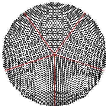
**Figure 9.** Reflector design, illustrating the cable structure's five axis symmetry
