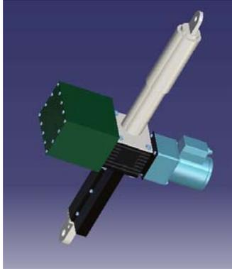
**Figure 12.** Illustration of a layout actuator design
