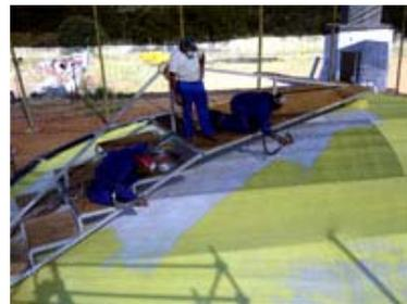
**Figure 26.** Flame-spraying the mould
