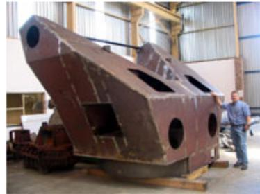
**Figure 22.** Manufacturing of the yoke
