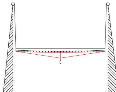
**Figure 11.** Reflector panel hanging from 3 towers
