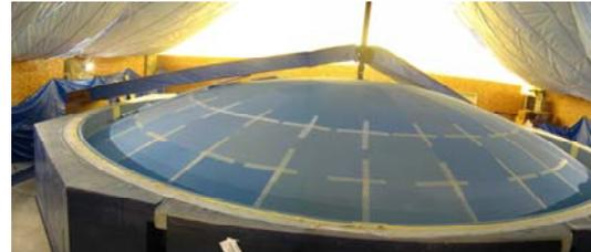
**Figure 6.** The reflector surface of the 10-m prototype laid in the mould. The blue material is foam core.
