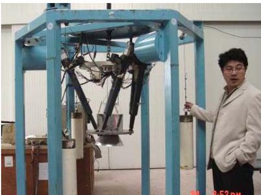
**Figure 13.** Experiments are conducted on the secondary stable platform of the FAST model's feed suspension system. Excellent vibration curbing effects have been achieved.
