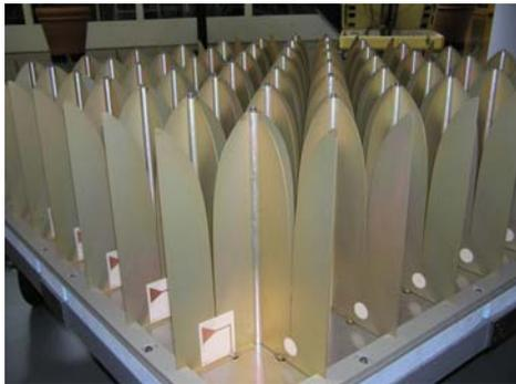
**Figure 17.** Another solution under development at ASTRON has the Vivaldi feeds as self-supporting solid structures made of anodised aluminium.
