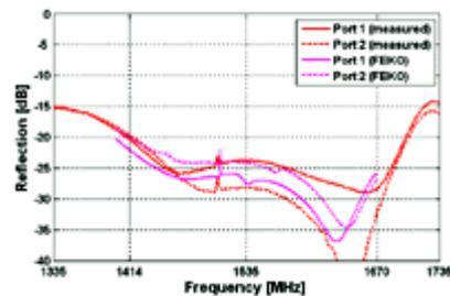
**Figure 33.** The predicted reflection coefficients agree quite well with the measured values - including the frequency of the trapped TE<sub>21</sub>L mode resonance. This resonance is caused by the asymmetry of the feed pin and was not apparent in initial coarser frequency sweeps. With the insight derived from this prototype and the agreement with numerical analyses, the next step is to remove the resonance.
