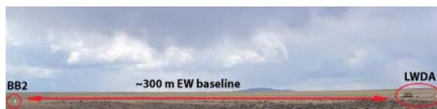
**Figure 40.** The LWDA interferometer. This two-element interferometer consists of the LWDA itself and a second-generation dipole (BB2) on a 300-m baseline. It is intended as a testbed for both antenna performance and software development.
