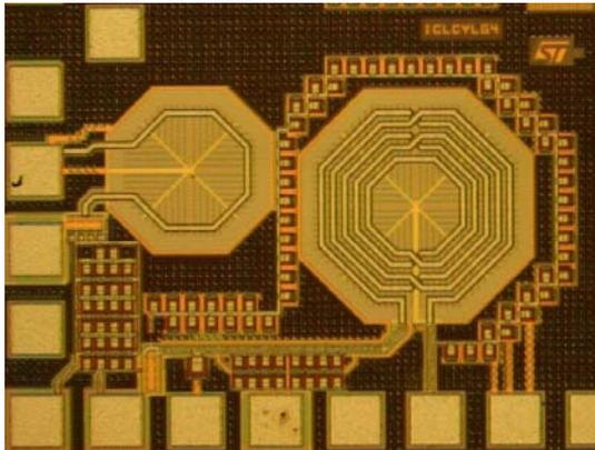
**Figure 5.** Die photo of a CMOS LNA that has attained a noise figure of less than 14K between 800 and 1500 MHz. The actual size of the device is approx 1mm.
