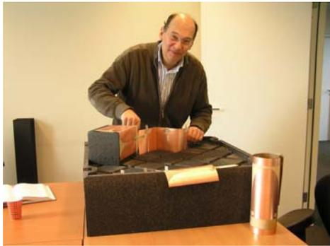
**Figure 16.** Arnold van Ardenne demonstrates one of the potential technologies for aperture-array tiles under development at ASTRON. The primary radiators are Vivaldi feeds printed on flexible circuit board and inserted into a foam support structure.
