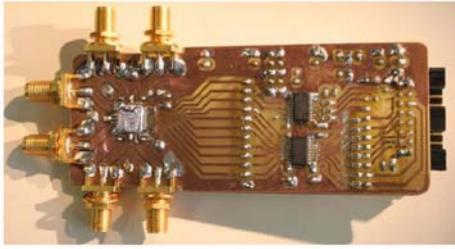
**Figure 15.** The beamformer chip developed in Nançay is shown here in its test module.
