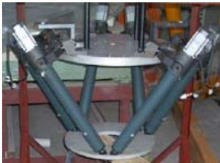
Fig.3. the new Stewart platform used for the Miyun FAST model
