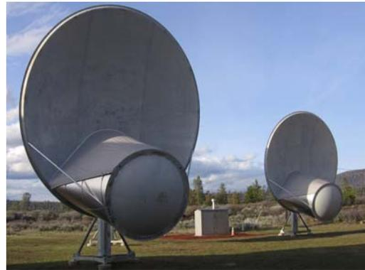
Figure 1: Two of the ATA dishes showing the near-final assembly, including the feed shroud in place.
