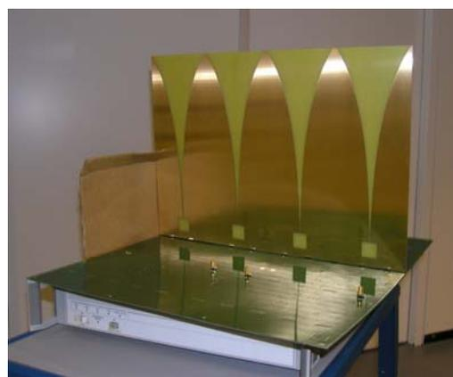
*This is a picture of Vivaldis designed for the prototype tile. Both RF circuit board and the antenna are shown.*
