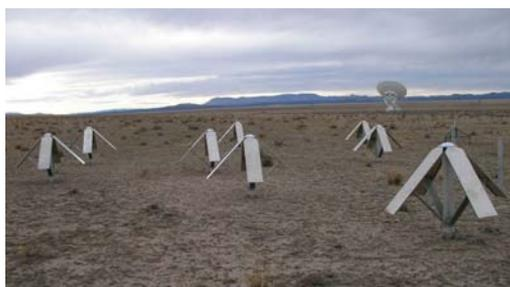
*Figure 3: The original eight dipoles of the Long Wavelength Demonstrator Array as deployed at the VLA site. (A VLA antenna is visible in the background.) Their locations relative to each other represent locations selected so that the full LWA station sidelobes are optimally low.*
