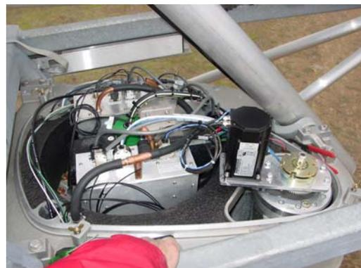
Figure 2: The azimuth drive (lower right), the drive electronics (lower middle), and antenna controller (middle) inside an ATA antenna alidade. The drive electronics box and controller box are field-replaceable units, needing only to undo a few connectors on the top. The black hose handles cooling air. The front-end is separately monitored and controlled—only 120V and fiber for the front-end pass through here.
