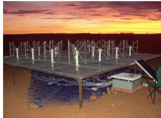
*Prototype dipole antennas of the Mileura Wide-field Array Low Frequency Demonstrator*
