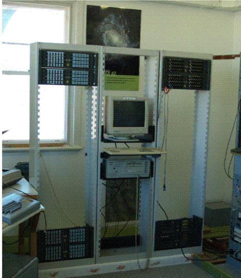
*Racks installed for panels, filterbanks, and correlator*
