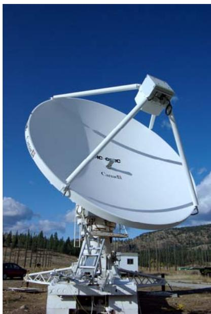
**Figure 6.** Is this what an SKA dish will look like? The 10-m Mk2 CART reflector with the PHAD phased-array demonstrator feed at the focus that were completed by NRC-HIA DRAO in Penticton during in October 2008.
