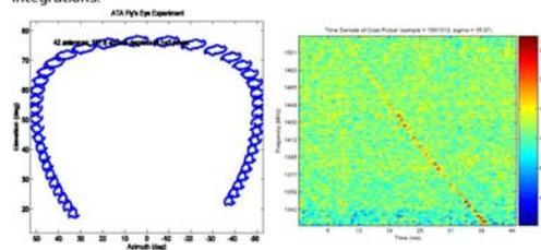
**Figure 24.** Bottom: Fly's Eye experiment: (left) positions of 42 antennas; (right) Crab pulse
