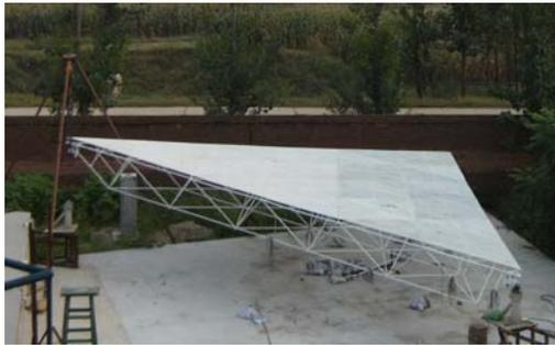
**Figure 11.** The 1-1 scaled reflector unit of FAST prototype
