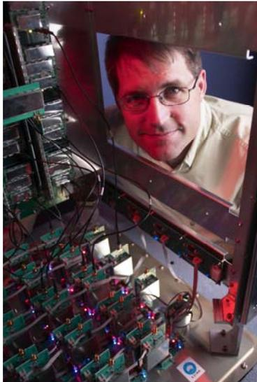
**Figure 2.** ASKAP Theme Leader Dave DeBoer with prototype receiver for the Parkes testbed focal plane array
