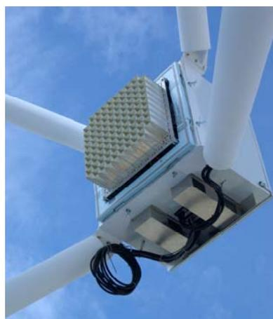
**Figure 7.** PHAD at the focus (radome removed)
