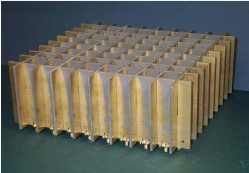
*Broad band, dual polarization array antenna designed for THEA demonstrator project.*
