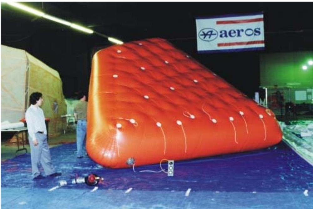
*Figure 2. Inflation Test of Tail Section of the Aerostat that will be used for field tests in Penticton*
