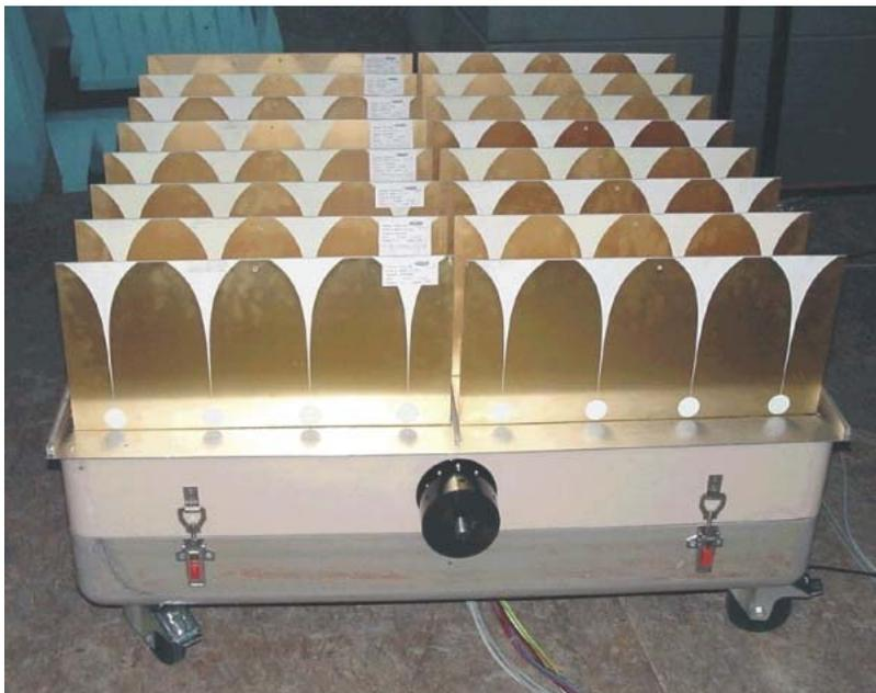
Figure 3. View of a Single THEA Tile with the radome removed.
