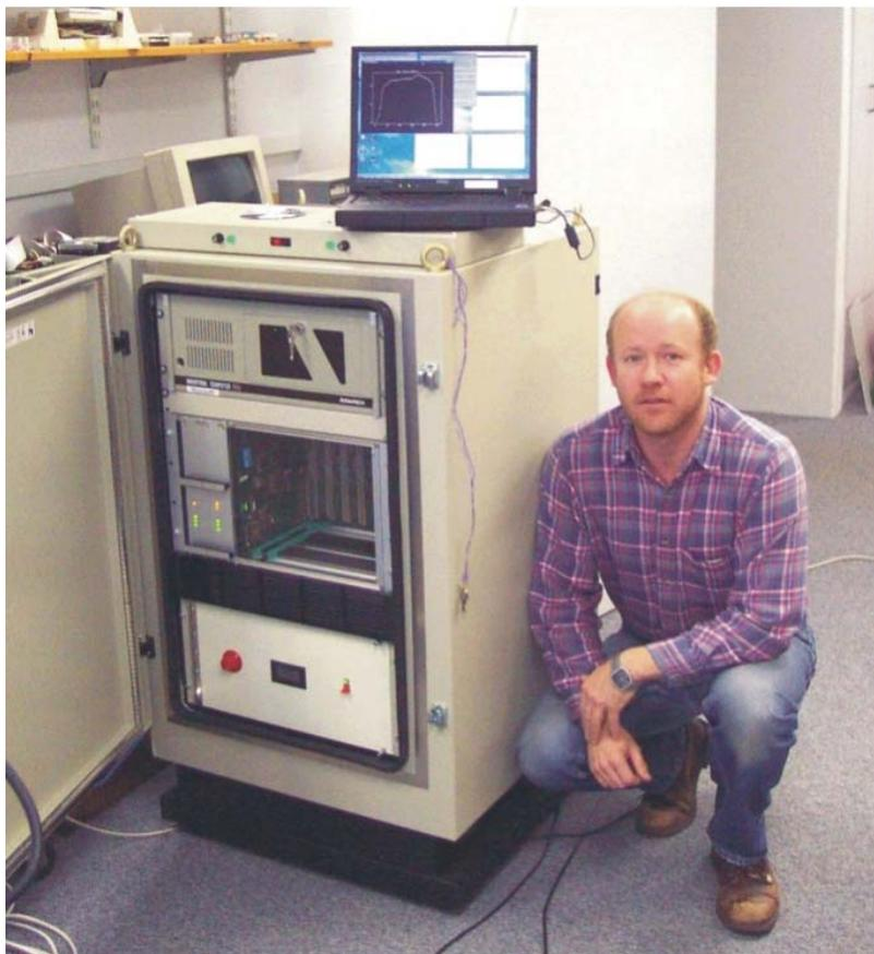
*Figure 1 - ATNF engineer Mal Smith with part of the high-sensitivity RFI measurement system he has constructed for use in SKA site tests and observatory monitoring roles. The auto-correlator (centre unit in rack) has a maximum bandwidth of 64 MHz (at 62.5 kHz resolution). With*
