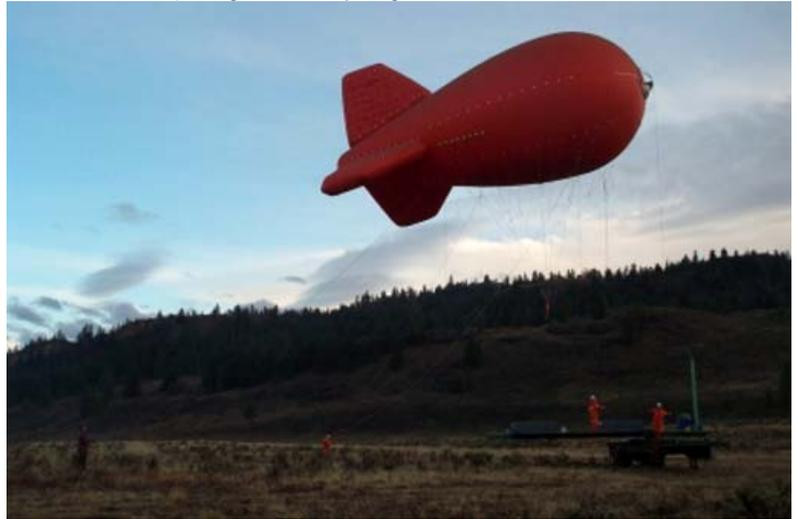
Figure 1. Retrieving the aerostat.
