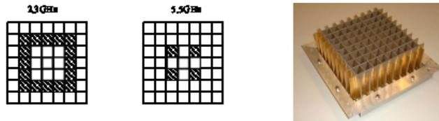
Figure 5. Sketch of the combined rings and a picture of the vivaldi array.
