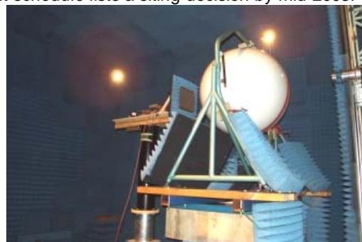
*8 x 8 THEA-style Vivaldi phased array (provided by ASTRON and MIT) being used as a focal surface array for a 0.9 m Luneburg lens. The array and lens combination were recently tested by CSIRO in its near-field test facility in Sydney; results will be available shortly.*
