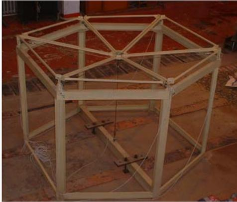
*Fig2a FAST cable-mesh reflector:
