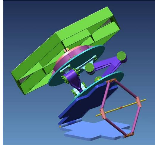
*Fig1b. The CAD map of Sarrus mechanism*
