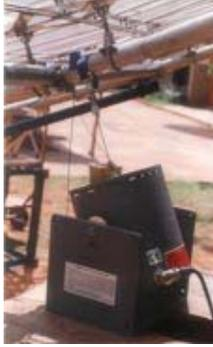
*Test setup for modal analysis showing the shaker*
