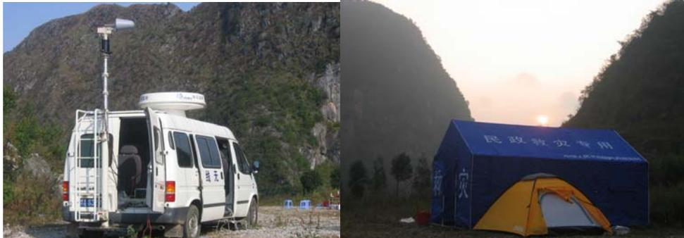
*Fig.4 Observations at Shangjiachong depression in Puding county during Nov.3-15 in 2004: A log-period antenna (HL050) equipped on the RFI monitoring van (left), plus two accommodation tents (right).*
