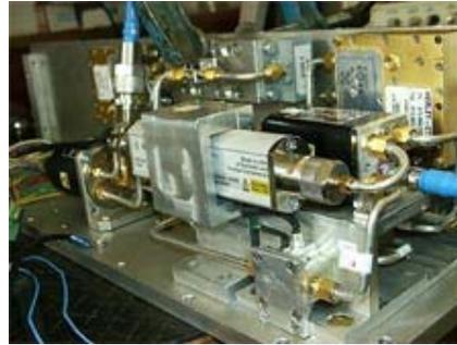
*Close-up image of the components and "plumbing" in the masthead unit.*
