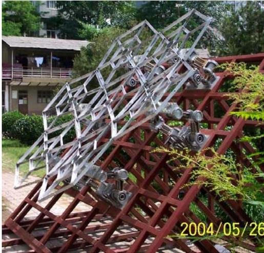
*Fig1a. A model of a Sarrus supporting reflector*
