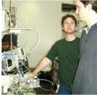
*Japie Fourie and Paul Manners checking the masthead unit that contains LNAs, mixers, local oscillators, noise diode and support electronics*
