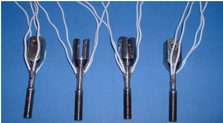
*Fig. 3 Force sensors made for the cable strain measurements by FAST group in HIT.*
