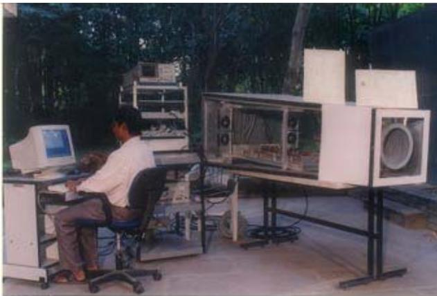
*A single polarization 4 to 8 GHz front-end receiver being characterized in the field. The testing of the control system has been completed. To provide redundancy and flexibility in the system, we have investigated two approaches, one using a Programmable Multi Axis Controller (PMAC) and the other using a LINUX-based PC.*
