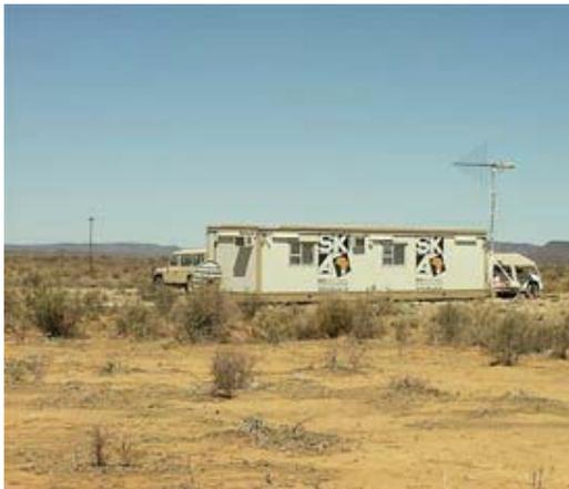
*View of the mobile office at the RFI measurement site on the farm Losberg. The antenna and mast assembly for RFI measurements is visible to the right of the container.;*
