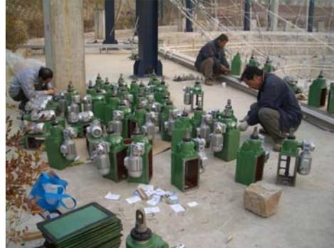
*Downward actuators to pull cable-mesh structure.*
