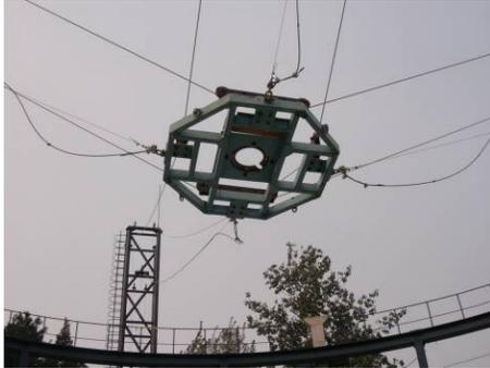
*The cable-car driven system for the focus cabin*
