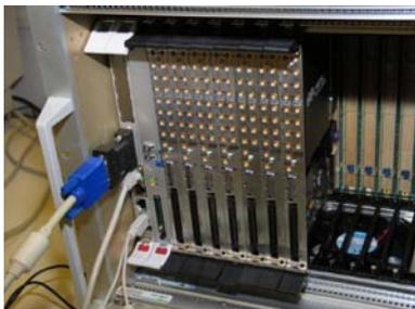
Figure 2. The commercial digital acquisition system being used in PHAD. Seven cards, each with 16 input channels, and 105 MSamples/s at 14 bit resolution are shown. Each card has 128 MByte RAM and an onboard FPGA. The complete system has 12 cards, giving 192 channels.
