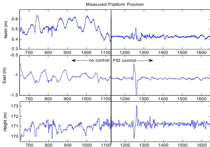
Figure 1. Confluence point motions with and without active tether control. Active control was switched on at 1125 seconds. The perturbation at 1250 seconds is a software glitch. The mean wind speed during the test was 4 m/s.
